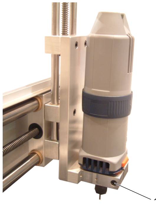
Illustration No. 12: Tool holder at Z-Slide (example: milling motor)
